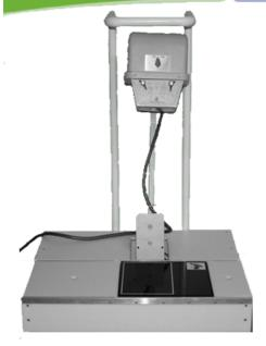
21 mega-pixel RAW Data resolution (4024×3016 true pixels) 8" x 12" Field of View.
